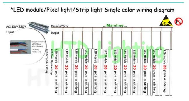
\*This product the most can tandem connection 20pcs module/50pcs pixel/5M strip, Prohibited beyond tandem connection. The thickness of power should according to actual possible present maximum current, the power of products, wiring length (suggest not exceeding 6M) and low voltage transmission line voltage drop.In measuring power use number of circumstances, should retain 20% of the allowance.
