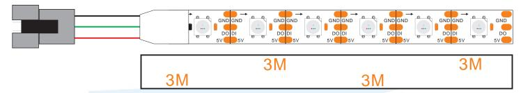
Pull the 3m paper out of the back of led strip
