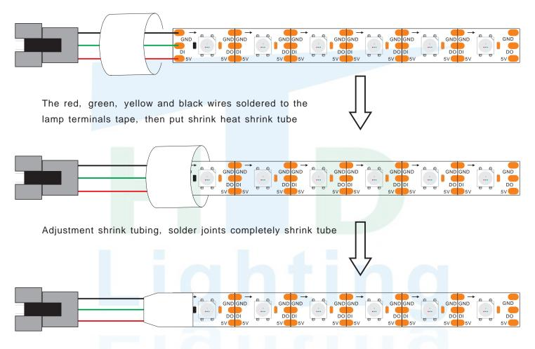
After adjustment shrink tube with hot hair dryer blowing shrink sleeve, shrink wrap the joints until completely
