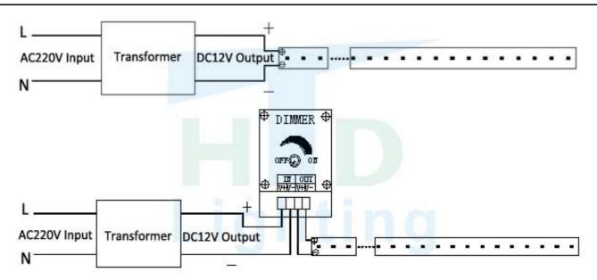
\*LED module/Pixel light/Strip light Single color wiring diagram
