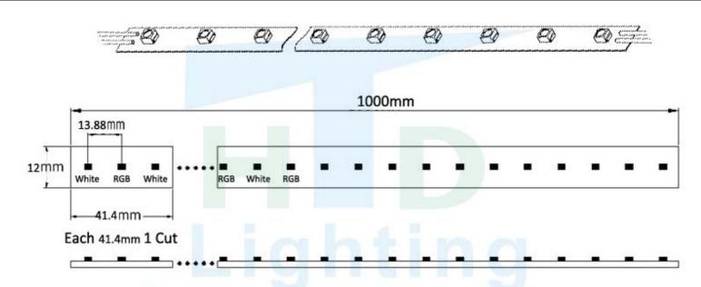
\*Note:IP20 Height is 1.9mm/IP65 Height is 2.9mm/IP68 Height is 3.9mm
